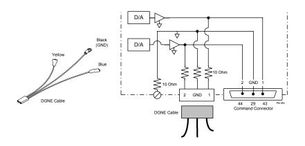
Figure 33: Diagnostic Cable (DGNE) Diagram
